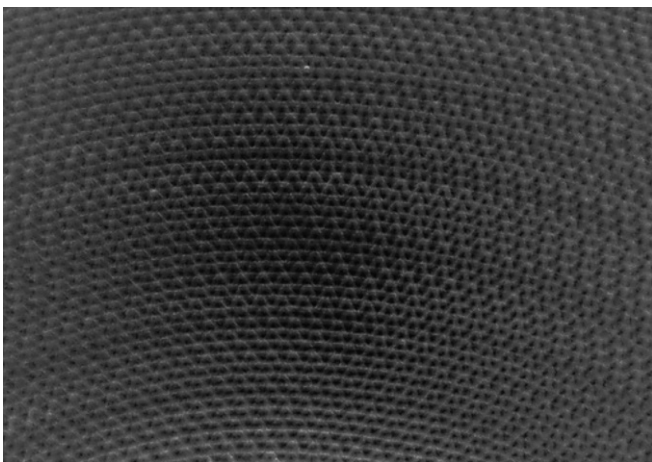
Fig. 2. Photograph of a portion of a total energy wheel showing the trapezoidal cross sections of the flow passages.
